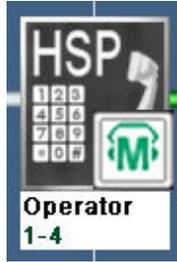
*Figure 2-6 This HSP is Monitoring Modules 1 Through 4*
