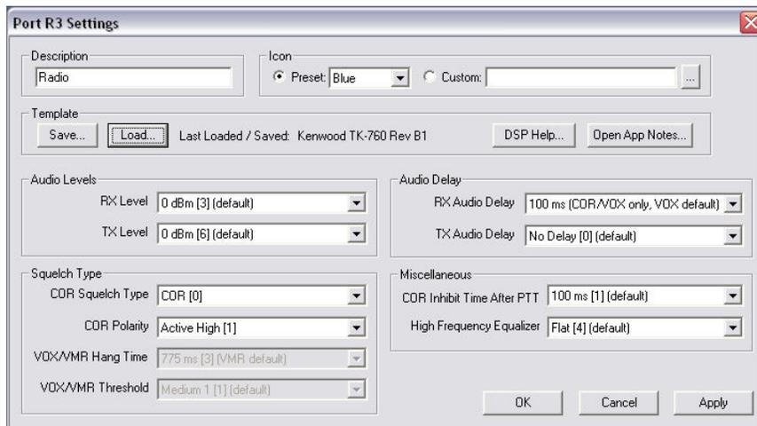
Figure 3-1 ACU-M Radio Port Settings Screen
