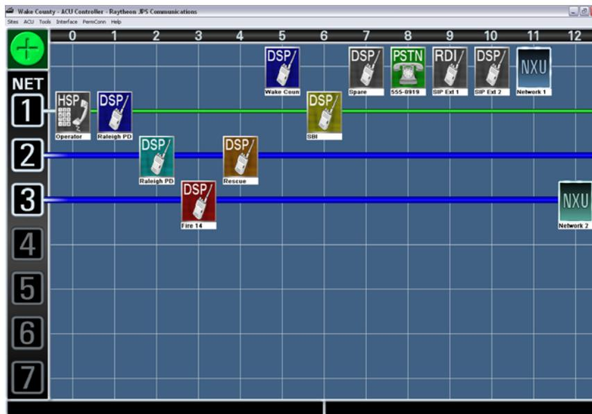
Figure 2-4 Nets 2 and 3 in a Vertical Connection
