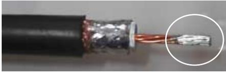
11. Insert the cable in the M-P connector as far as it will go.
