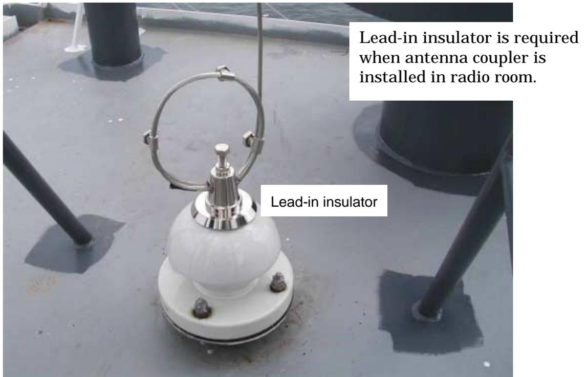
*Fig. 3-5 Antenna lead-in insulator*
