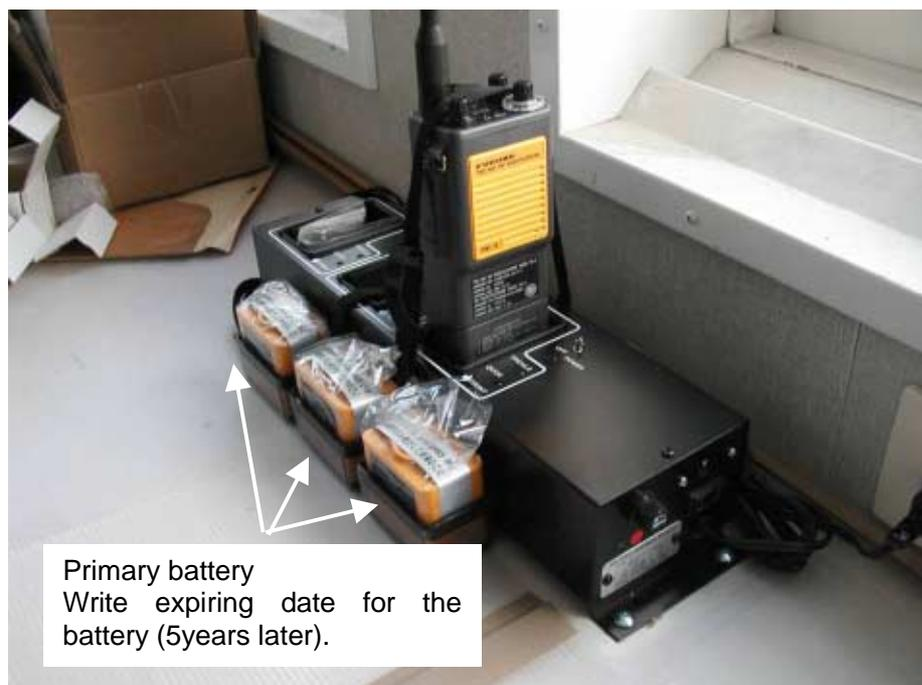
Fig. 3-35 Primary batteries
