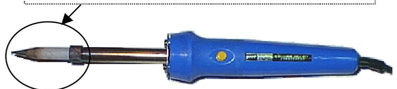
Example 15 to 150 W adjustable soldering iron
