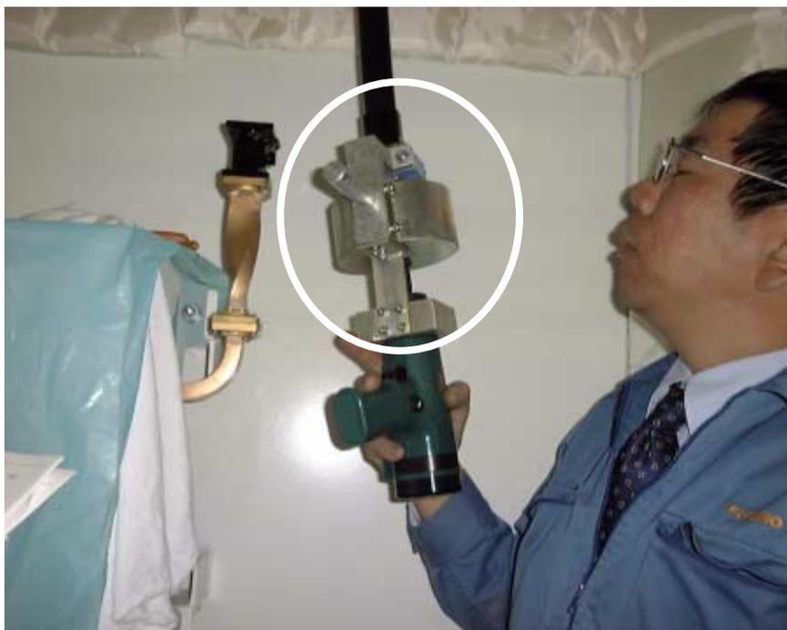
Fig. 1-20 Widening waveguide opening
