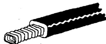
Finish the edge of the conductor with a file.
