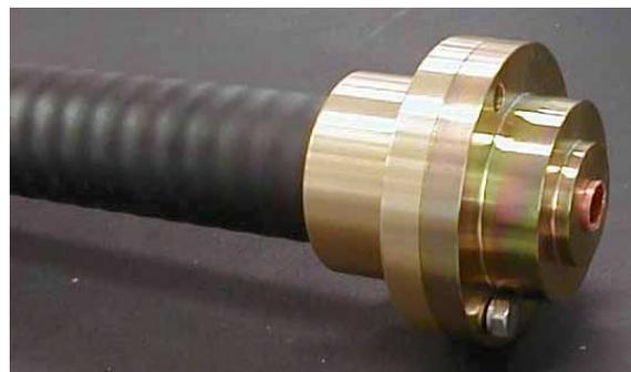
10. Remove the gauge. Then, file the inner conductor to finish.
