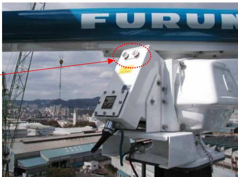
Fig. 1-8 Performance monitor on X-band scanner unit
