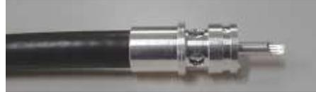
12. Solder the connector and shield through holes.
