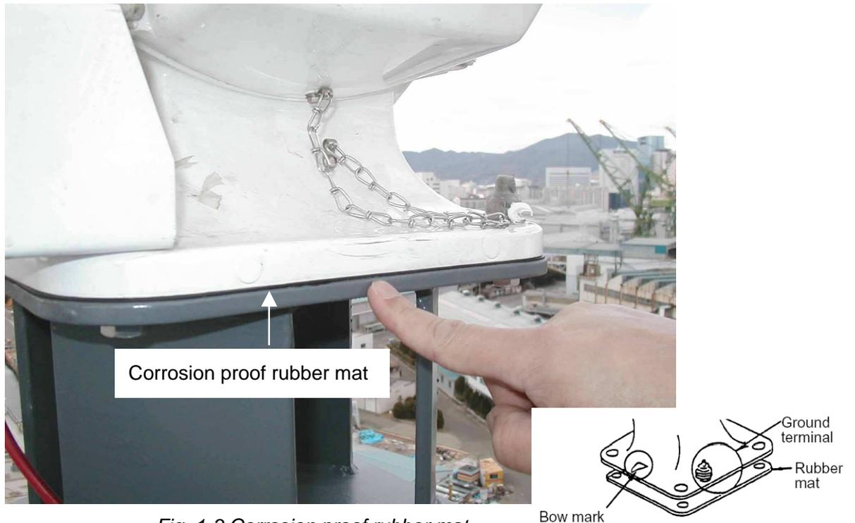
Fig. 1-3 Corrosion proof rubber mat
