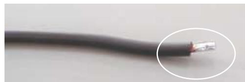
5. Apply a thin layer of solder to the tap.
