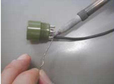
8. Use the right amount of solder. Do not move parts until the solder has cooled.
