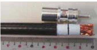
7. Remove the shield from the mark.
