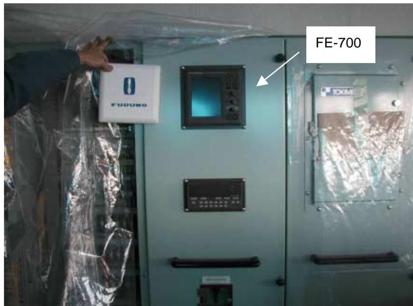
Fig.5-48 Installation of FE-700 echosounder
