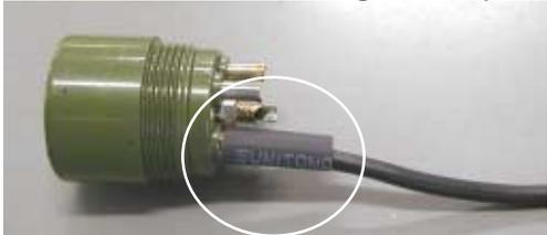
10. Heat the tube by the soldering iron.
