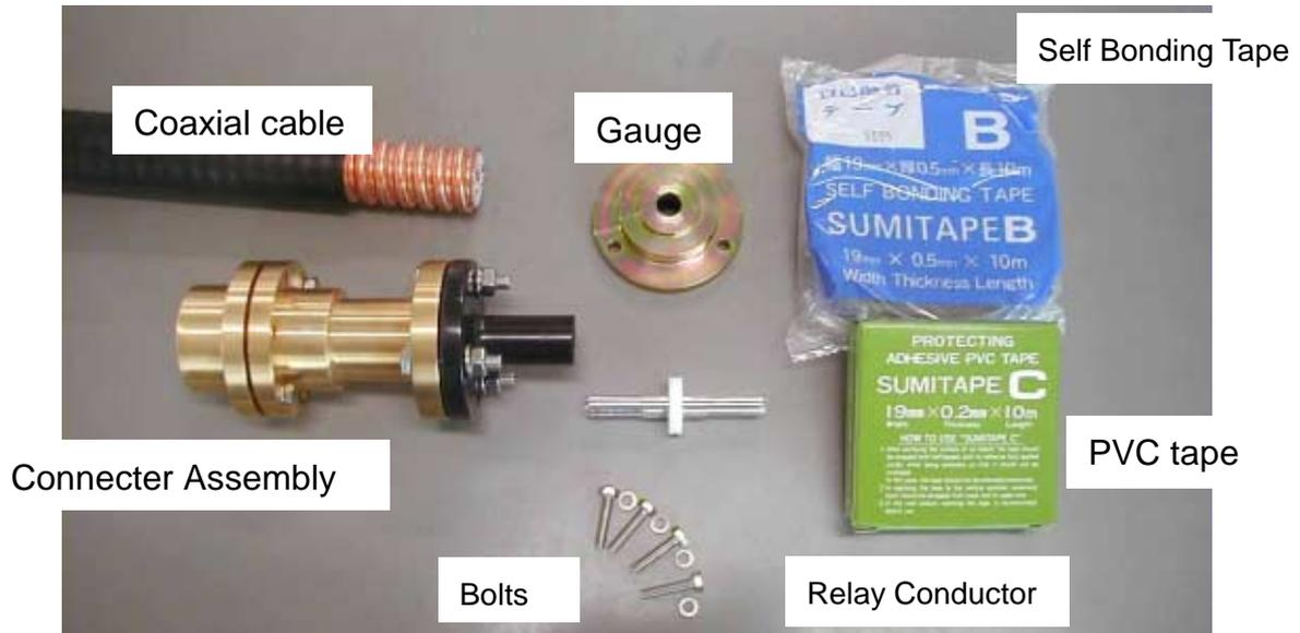
Note1: Prevent foreign substances from being entered into the cable during the work.
