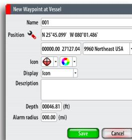
You can position a waypoint at the cursor position on a chart, radar and echo sounder panel by moving the cursor to selected position and then pressing the **PLOT** key.
