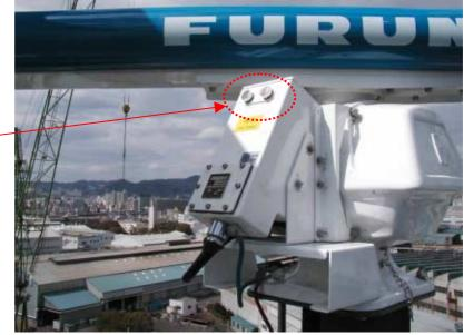
Fig. 1-8 Performance monitor on X-band scanner unit
