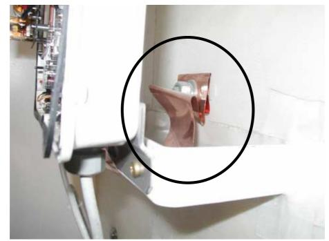
Fig. 3-10 Grounding antenna coupler
