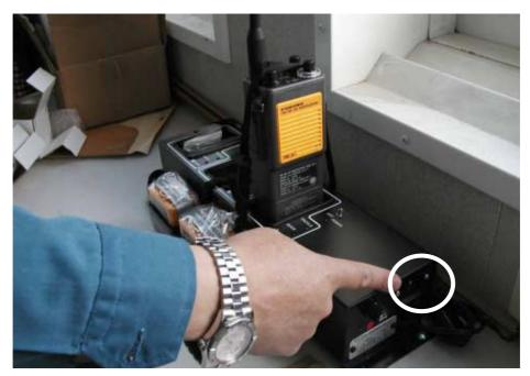
Fig. 3-34 Two-Way Radio charger
