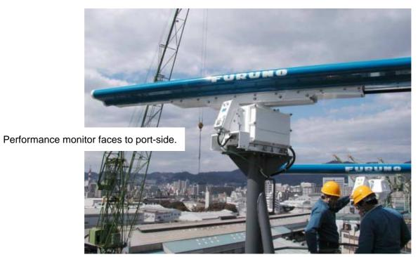
Fig. 1-13 S-band scanner unit with performance monitor fitted.
