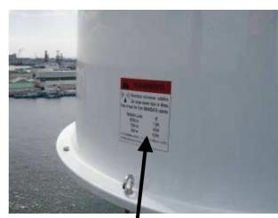
The label on the radome tells safety distance. Fig. 2-5 Radio frequency radiation hazard label
