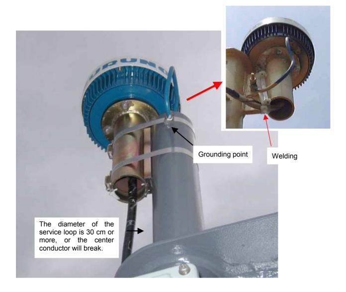
Fig. 2-6 Inmarsat C antenna unit
