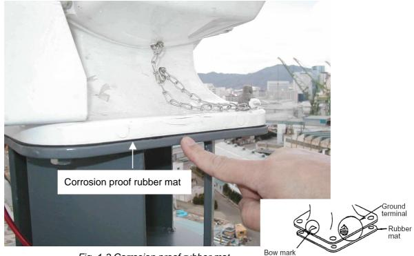
Fig. 1-3 Corrosion proof rubber mat
