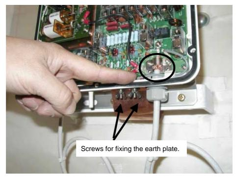
Fig. 3-11 Connecting copper plate to antenna coupler
