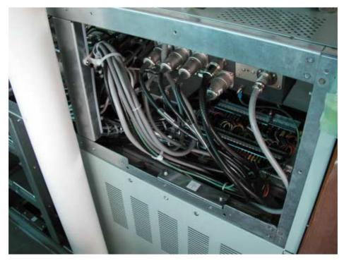
Fig. 3-23 RC-1800F with rear panel removed
