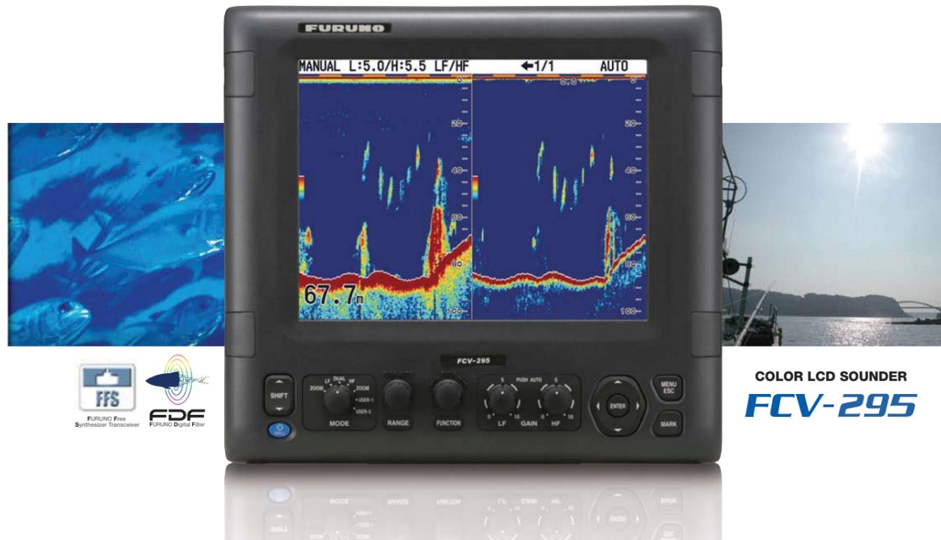
The FCV-295 is a new color digital sounder designed for a variety of professional fishing operations. It features a bonded 10.4" LCD display providing superior viewing even in direct sunlight. You can display echoes in 8, 16, or 64 colors, with color assignment dependent on the strength of the returned echo.
