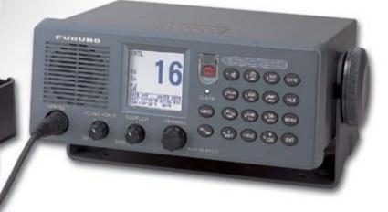
The FURUNO FM-8800S/8800D are high quality, all-in-one marine VHF radiotelephones designed to comply with the GMDSS carriage requirements for safety and general communications. All the necessary functions such as a 25 W VHF radiotelephone, a Class A DSC modem and a CH 70 Watch Receiver are incorporated into the compact transceiver unit.
