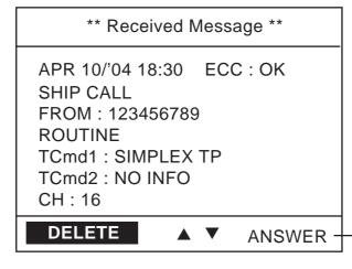
For a received message which requires a reply, ANSWER is displayed (for 4.5 minutes). To reply choose it and press the **ENT** key.
