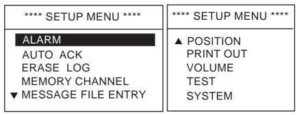
2. Rotate the **CH** knob (or press up / down arrow key) to choose SYSTEM from page 2 of the menu and press the **ENT** key. The following window appears. The self ID is displayed on the first line.
