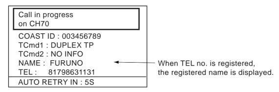
If a response from the coast station is received within five seconds, transmit PSTN CALL (EOS) signal and then carrier frequency during two seconds. Then your phone rings. Press the **CANCEL** key to stop the calling sound and change to standby display. Hook off and communicate with other party.
