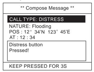
The distress alert with nature of distress, ship's position and time are transmitted. The sequence of display and procedures are the same as in paragraph 2.1.
