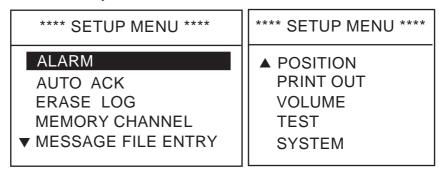
2. Rotate the **CH** knob to choose SYSTEM and press the **ENT** key. The following selection window appears.
