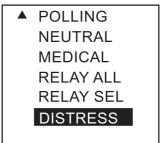
3. Rotate the CH knob (or press up / down arrow key) to choose DISTRESS. Press the **ENT** key.
