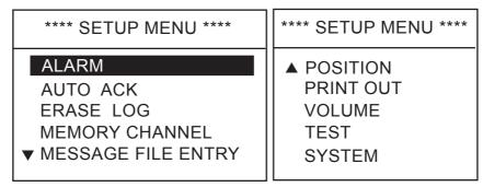
2. Rotate the **CH** knob (or press up / down arrow key) to choose SYSTEM from page 2 of the menu and press the **ENT** key. The following window appears.
