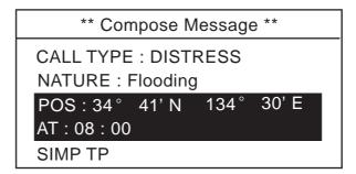
The own ship's position and current time in UTC are displayed if your FM-8800D/S is connected to a navigation equipment, for example, GPS.
