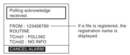
Press the **CANCEL** key to silence the alarm. Press the **ENT** key to show the standby display when you can confirm if called party is within communicating range.
