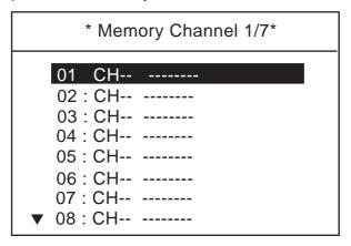
Rotate the CH knob (or press up / down arrow key) to choose a vacant CH number and press the ENT key.
