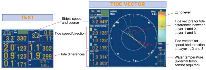
Tide speed and direction for the three depth layers are displayed with vectors. The depth of each layer can be set manually in 1 m intervals. Other information such as tide differential between the reference and one of the two other layers, heading and course can also be displayed in large text.
