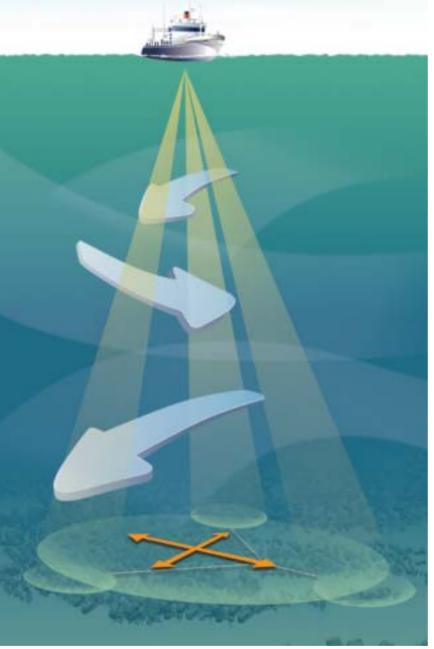
The FURUNO CI-68 is a new Doppler Sonar Current Indicator designed for various types of fish and hydrographic survey vessels.
