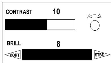
2. Press the [PORT] or [STBD] key for adjusting BRILLIANCE. Rotate the [ENTER] knob for adjusting CONTRAST.
