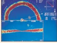
the mode integrating the two images shown to the left. This sonar image also can be switched to a Half Circle with Vertical scan.
