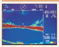
The vertical scan paints the bottom profile within a user-specified vertical plane. The cursor indicator reads slant range and soundome tilt.
