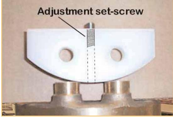
Please confirm that the narrowest gap between the tank guides and the retraction tube wall is **0.5mm**. Adjust if necessary.
