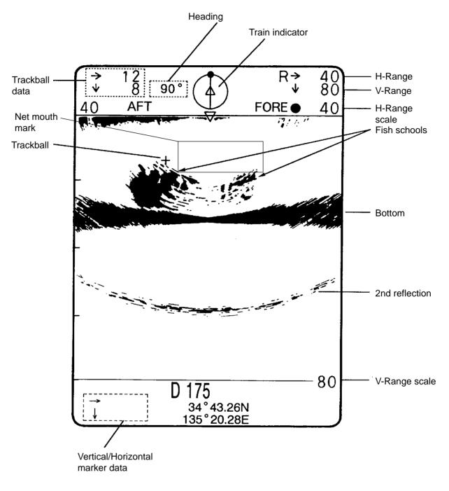
Figure 3-15 Indications in the vertical fan mode
