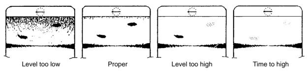
Figure 3-8 Examples of proper and improper TVG
