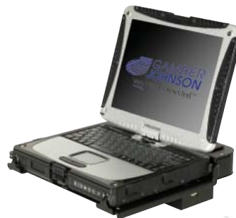
Easy-to-use "lift-and-turn" compression latch
