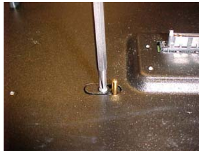
Single Cap positioned to block WLAN contact
