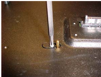
Single Cap positioned to block WLAN contact
