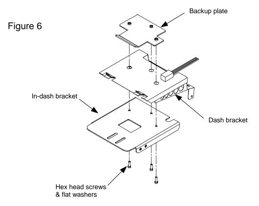
After assembly of the In-Dash Bracket is complete re-assemble the Heater Control Panel from Figure 3, re-connect the Wires for the Truck Release from Figure 3, and re-attach the Dash Trim Panel from Figure 2.
