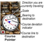
The course pointer provides an indication of drift (right or left)
