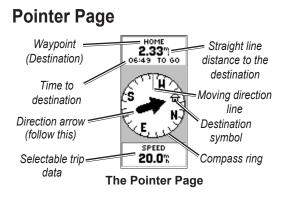
The Pointer page helps guide you to a destination. When navigating towards a destination, the Pointer page shows the name, the distance, time to go, and a direction arrow in the compass ring.
