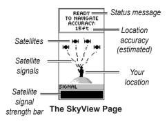
The SkyView page displays the GPS receiver status. It also shows the strength of the satellite signals. A READY TO NAVIGATE message is shown when the receiver has gathered enough satellite information to begin navigation.
