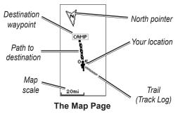
The Map page shows where you are located, and as you travel, the animated figure leaves a track log. The map also shows waypoint names and symbols. The eTrex is set to automatically rotate the map as you move, so waypoints that are ahead of you are always displayed in front of the animated figure. The map orientation is shown in the upper left corner.
