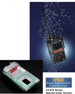
For even more demanding environments, the VX-870 Series version meets IP68 specifications (submersion to 6 feet for 3 hours), and is available via special order.
