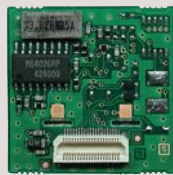
FVP-36 Inversion Encryption Unit (VX-920/970)
