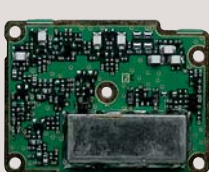
SRX-4 Multi Band Receiver Unit (134-174 MHz)
