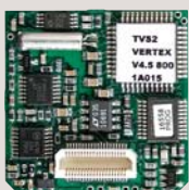
FVP-35 Rolling Code Encryption Unit (VX-920/970)
