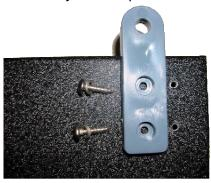
Ensure that all screws are fully tightened. The heads of the screws should be fully recessed into the cavities in the feet, so that the screws will not touch the mounting surface of the vessel.
