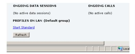
If a primary profile is already active, your new profile will not appear as a link but as plain text. The active primary profile is displayed as a link with the text "Stop <name of profile>". Click this link first to stop the active profile. Then click your new profile, which is now displayed as a link.
