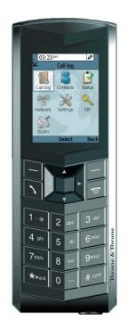
When connected to the terminal the IP handset provides a dedicated BGAN menu with a subset of the terminal configuration options.
