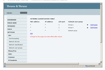
The network classification table shows which devices are associated with which LAN ports and network user groups. An Asterisk (\*) is a "wild card", meaning that any value is accepted.
