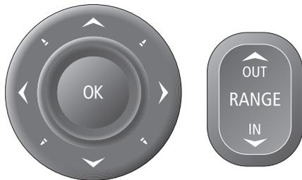
To move around the chart and display the area required at an appropriate scale, use the track pad and range in/out buttons.
