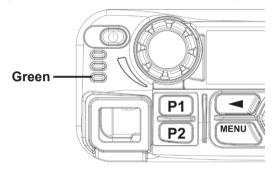
**NOTE**: The green LED lights up while the radio is transmitting and blinks rapidly when the radio is receiving a privacy-enabled call.
