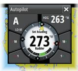
Adjust set heading (Auto mode), set wind angle (Wind mode) and set course (NoDrift mode) by tapping the **Port** or **Starboard** buttons in the autopilot pop-up. Heading can also be adjusted by tapping the HDG button and entering a heading value.
