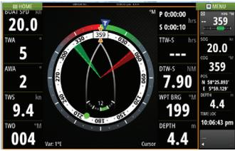
SailSteer provides a composite view of key sailing data. All data is displayed relative to the yacht's bow. The number of data fields included in the panel is dependant on available panel size.
