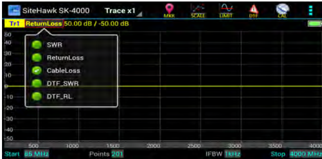
Figure 10 Selecting Cable Loss Measurement
