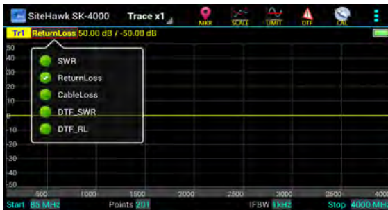
Figure 8 Selecting the Measure Match Mode
