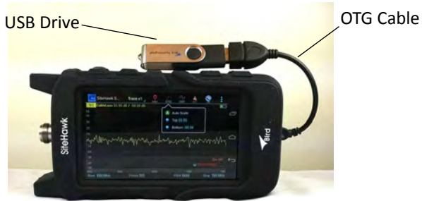
Figure 48 USB Drive connections
