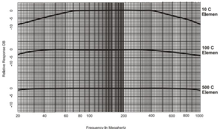
These curves are typical for all element types (H, A, B, C, D, ...) at their respective frequencies. Since a C type element has a frequency range of 100 - 250 MHz, response curves for other element types can be approximated by replacing the 100 and 250 MHz points on the chart with the extremes of the element's frequency range, and recalculating the other frequency points accordingly.
