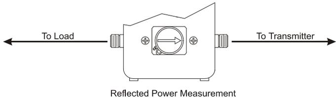
When readings are being made with the wattmeter connected to an auxiliary RF line section, do not put an element in the unused line section. Otherwise, the DC circuit will be unbalanced or shorted, causing inaccurate or zero power readings.
