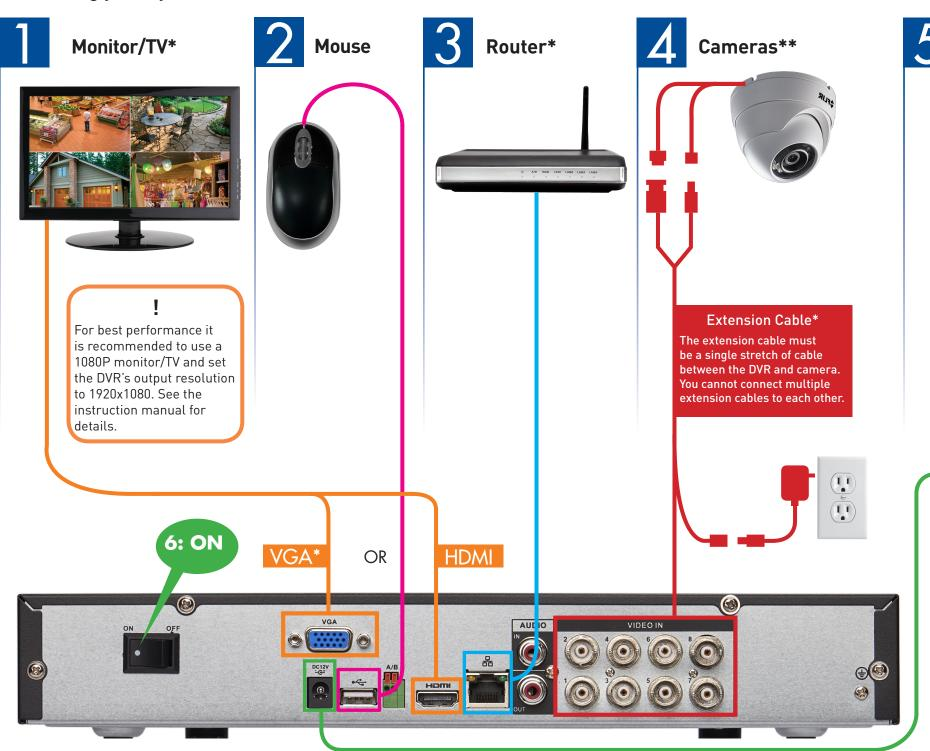
8 channel configuration shown. 4/16 channel will have the respective number of video inputs.
