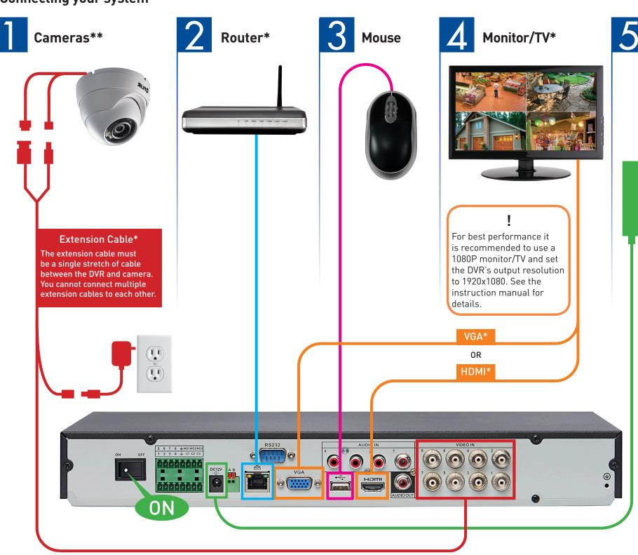
8 channel configuration shown. 4/16 channel will have the respective number of video inputs.
