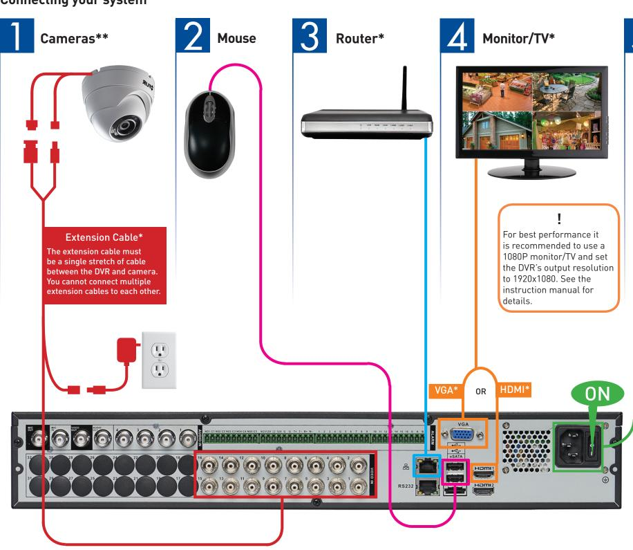
16 channel configuration shown. Other channel configurations will have the respective number of video inputs.
