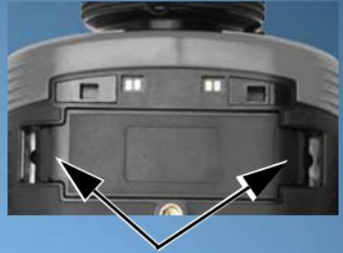
Grasp spring loaded buttons on SD card door edges and pull
