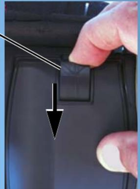
5. Snap the SD card door back into place and re-install the battery cover—it only fits one way.
