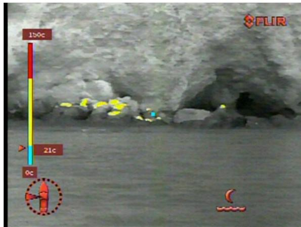
**Tracking.** When tracking is enabled, you manually identify an area on the screen that you want to track and then engage the tracker. The tracker keeps the camera pointed toward that target area. You can fine-tune the target area and make other manual adjustments. This feature can be useful when rescue personnel are attempting to contact a vessel in distress or a person overboard. See “Using Voyager III Tracking” on page 33 for details.
