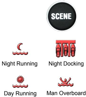
The preset AGC settings for each scene have been optimized to offer the most balance and high quality image for specific conditions. Which setting to use depends on personal preference and environmental conditions. You may like the way the Night Docking setting looks, even though you are running on open water during the daytime. Experiment with the different settings, and find out for yourself which settings works best in different conditions.
