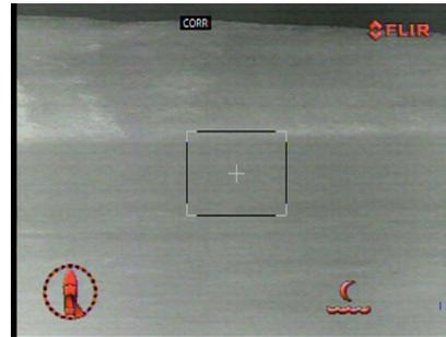
You should move the camera until the white tracking gate shows inside the acquisition window before attempting to engage a target. The tracker automatically sizes the white tracking gate as it finds a discernible target.
