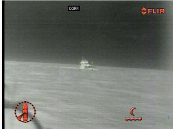
You can use firefighter mode and tracking mode together to provide comprehensive support for rescue operations. In the man-over-board scenario, you can use color coding associated with a temperature range to identify where the person is located and then engage the tracker to keep the camera focused on the person until the completion of a successful rescue operation.
