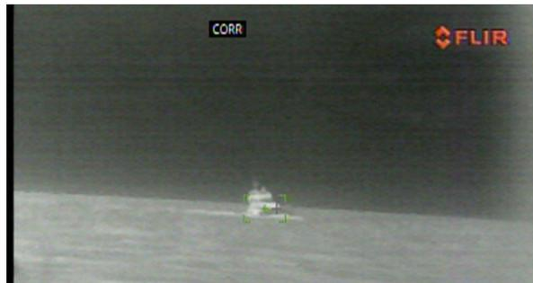
In this figure, the black acquisition window no longer displays, and the color of the tracking gate is now green, indicating that it is tracking the target area. The system displays gray cross hairs to marks the center of the scene. When the tracker is exactly on target, the green cross hair of the tracking gate overlay the gray cross hairs.
