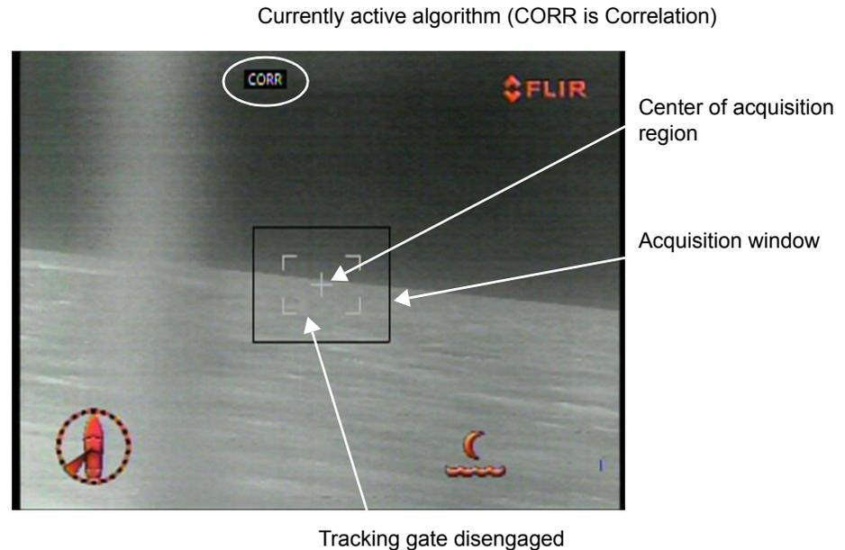
The letters at the top of the screen (CORR) indicate the method the system is currently using for acquiring targets in the region of interest. This method is called an acquisition algorithm, and you can select from four algorithms.
