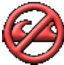
Select this option to enable or disable the two-axis mechanical gyro stabilization, which prevents camera images from being affected by mechanical vibrations caused by waves and ship motion. This setting is enabled by default and should not be changed under normal operation. The icon to the left flashes when you enable this setting but does not display continually since this is the normal mode of operation.
