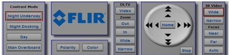
The red highlight around a particular control indicates the active setting. In this image, the wide FOV camera is displaying using the Night Underway contrast.
