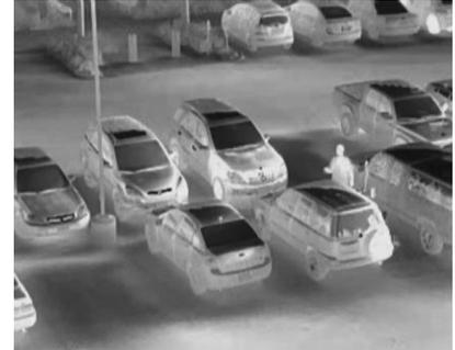
The possible color modes are configured on the System Setup Menu (see “Color Thermal Video” on page 50 for details). Use the Polarity button to switch between white-hot and black-hot:
