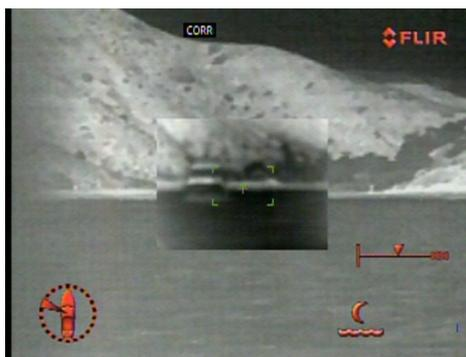
The Autofocus scale shows progress of the focus operation
