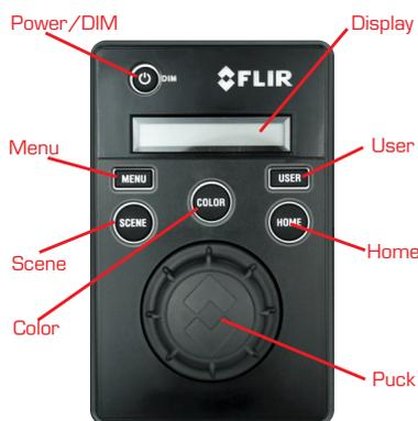
All of the buttons on the JCU perform multiple functions. In most cases, each performs one function when it is pressed briefly (short press) and a different function when it is pressed and held (long press). This flexibility enables a simple device to support a set of complex, rich features.
