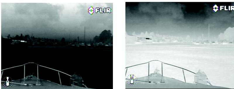
If Color Thermal Video is enabled, you have additional color choices. Inverting the polarity switches the darker and lighter colors.
