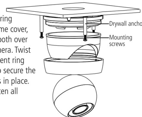
**G** Move the ball camera to the desired position. While holding the ball camera firmly in place, twist the adjustment ring the rest of the way to secure it to the camera base. Holding the camera prevents it from moving while securing the adjustment ring.
