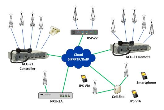
The ACU-Z1 and RSP-Z2 minimize BW required as well as maintain local interoperability in the event of an incident that causes a disruption to the network. Local links are created within the ACU-Z1 or the RSP-Z2, and maintained if a network outage occurs. Bandwidth is minimized because, rather than sending independent audio streams, the combined audio of the interoperability nets is passed to the controlling ACU-Z1.
