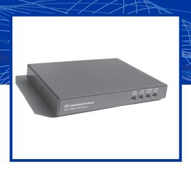
The ARA-1 extends the coverage and capability of an existing SIP PBX by allowing the interface of LMR radios to the system. It's comparable to an analog telephone adapter (ATA), which allows a standard telephone to operate on a SIP network; the ARA-1 provides the same capability to a radio.
