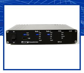
This versatile VoIP to analog interface allows a radio, a pair of radios, or a radio and a PSTN connection to be patched together and/or remotely interfaced to other devices or to a dispatch capability via various common protocols: SIP, RTP, or JPS RoIP.
