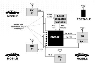
SNV-12 Voter system with 12 receivers; the RX signal from the receiver voted with the best audio is retransmitted by the Site 1 local transmitter.
