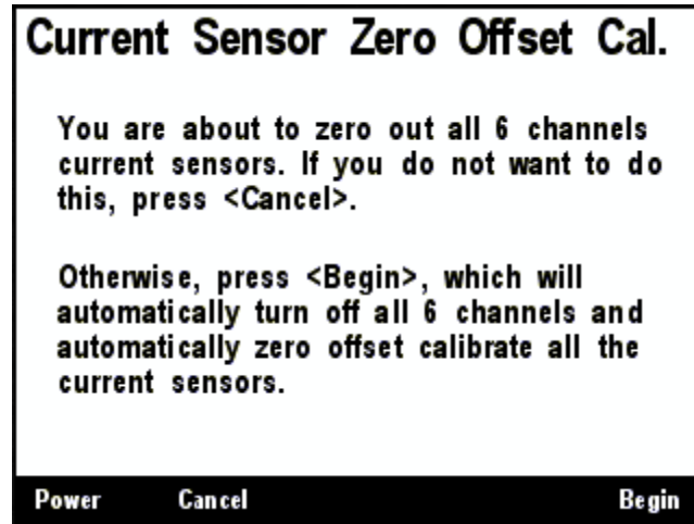
Figure 54 – DCR100 Current Sensor Zero Offset Calibration Screen
