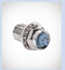
The Bulkhead Feed-Thru allows ease of installation through panels or bulkheads and establishes future connection points in a network installation. The bulkhead feed-thru also maintains the integrity of watertight bulkheads by providing a waterproof seal and connection.
