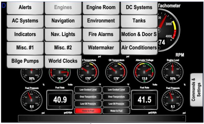
Figure 9 – N2KView<sup>®</sup> Window with Tabs Displayed
