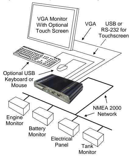
Figure 1 – MBB200C Network Diagram
