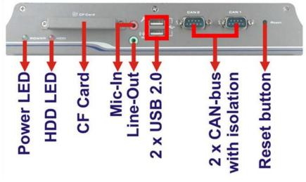
Figure 3 – MBB200C Front Panel Connections
