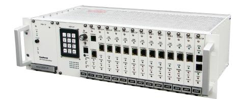
The SIP interoperability of the ACU-2000 IP gateway allows a remote user with access to a SIP device and network connection to communicate via radio from any remote location by simply dialing an extension. The ability to easily share critical information in real time helps better coordinate personnel and resources for a more effective response during routine activities and emergency situations.
