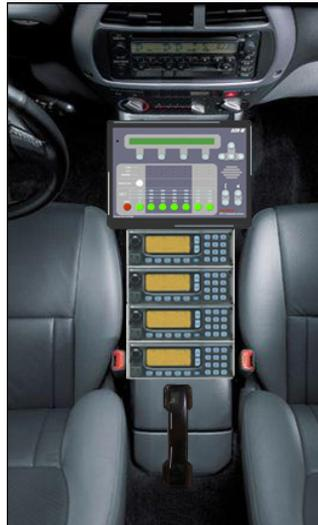
**Figure 24: ACU-M and Radios mounted in Center Console of a Sedan, Light Truck, or SUV**
