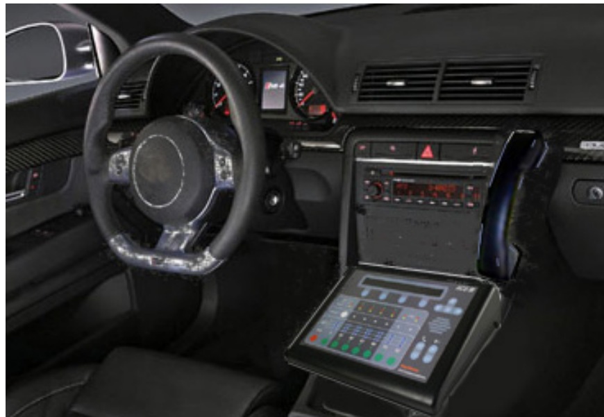
Figure 3: Typical ACU-M Vehicle Installation
