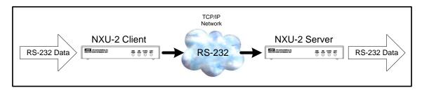
In conjunction with RS-232 data, the NXU will also simultaneously multiplex VoIP data within the same Ethernet data stream as the RS-232 data. This combination makes the NXU an ideal solution to control land mobile radio devices over the Ethernet, as will as support VoIP audio applications.
