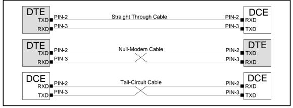
The following diagram illustrates how straight through and null-modem cables are specified when connecting devices to the NXU.
