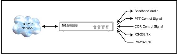
NXU units are network devices, meaning they can be identified over the network with unique IP addresses. Two NXU's in *Normal Mode* can be associated across a TCP/IP network by assigning
