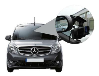
Clean the windshield with alcohol and make sure it is dry. Then remove the red 3M paper from the adhesive and press firmly and hold on the windshield for about 20 seconds.
