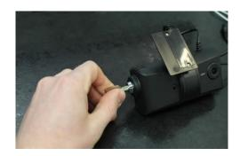
Adjust the angle of the bracket to the desired angle and slide in to lock in place. When you are happy with the angle on the windshield, slide the case back onto KP1 and lock.
