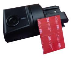
Apply both pieces of provided 3M adhesive to the mounting bracket and press firmly to adhere.
