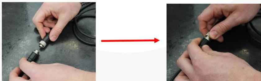
**To connect the cable to either the cigarette lighter adaptor or either junction box, attach by lining up the arrows on each cable and then push together. To secure them together, twist the silver plate as shown below.**
