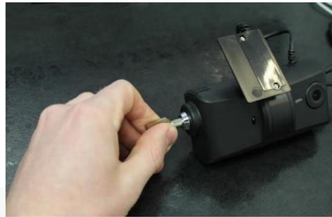
Adjust the angle of the bracket to the desired angle and slide in to lock in place. When you are happy with the angle on the windshield, slide the case back onto KP1 and lock.
