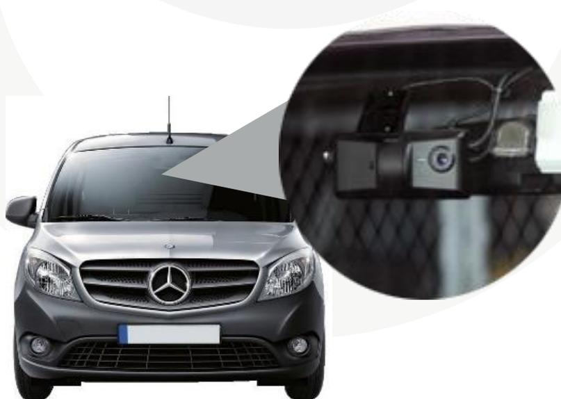
Clean the windshield with alcohol and make sure it is dry. Then remove the red 3M paper from the adhesive and press firmly and hold on the windshield for about 20 seconds.
