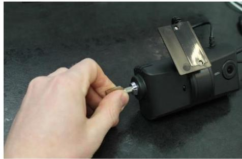
Use the provided keyset to unlock and remove the locking cover. To unlock the cover, insert the provided keyset and turn counter-clockwise 90 degrees. Once unlocked, press firmly on the two buttons on either side of the cover and pull the door away from the camera.
