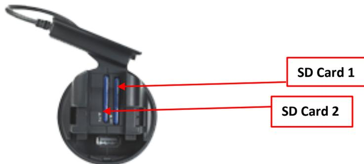
SD card(s) must be first initialized with KP1 Config Tool software, which is available for download on our website: <http://support.smartwitness.com> . After SD card initialization, you can customize your settings and save the settings to your SD card(s). The settings will apply to the camera at the next power up.
