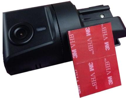
Apply provided 3M VHB adhesive pad to the mounting bracket and press firmly to adhere.
