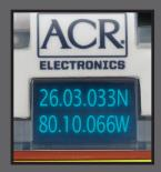
When activated, 406 MHz transmissions, usage tips, and the beacon's latitude and longitude are displayed.
