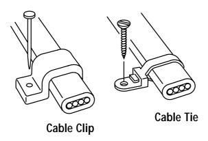
**Note:** Do not use metal staples or a staple gun to secure cables. Metal staples—especially when installed with a staple gun—have a tendency to cut the cables.
