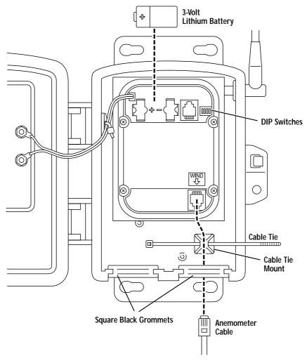
SENSOR INTERFACE MODULE ON ANEMOMETER TRANSMITTER
