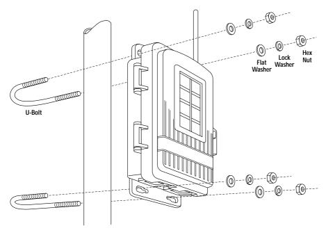
MOUNTING TRANSMITTER SHELTER ON A POLE
