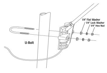
MOUNTING ANEMOMETER ON A POLE
