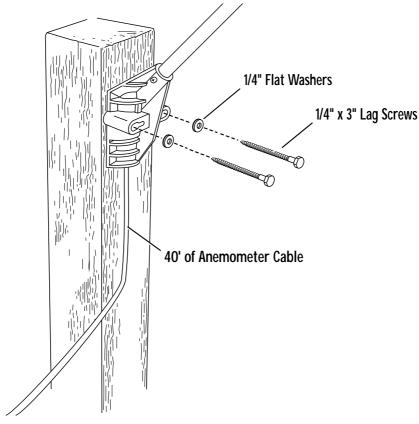
MOUNTING ANEMOMETER ON A VERTICAL SURFACE
